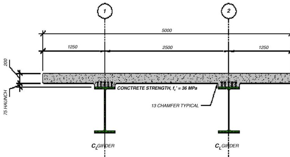
Fig. 2. Typical cross-section of bridge deck concrete details.
