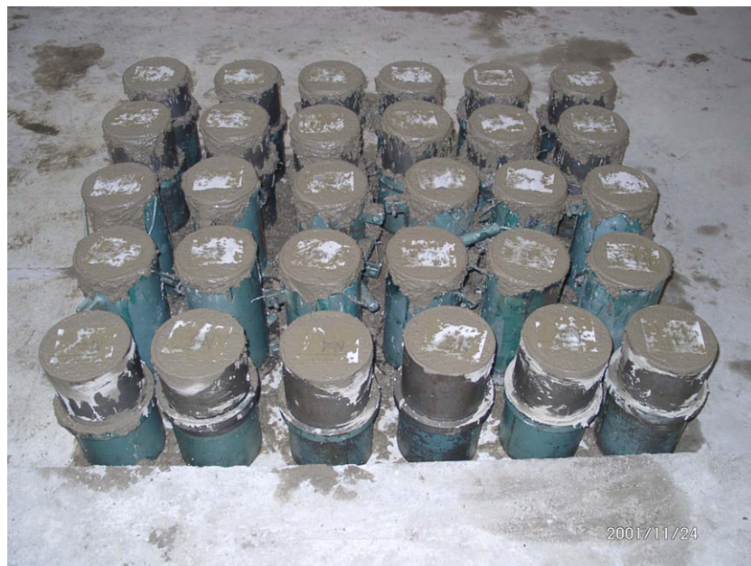
Fig. 1. Five different concrete batches, the first one being an ordinary C20 class without any SFs, and the other four containing SFs of varying dosages again in the same C20 class concrete.
