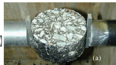
Fig. 2. Schematic of the SHPB apparatus and typical pulses obtained in testing (a) specimen configuration for dynamic IDT testing.
