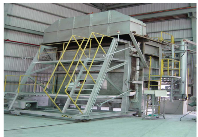
Fig. 1. The heavy-oil burning furnace at the Fire Protection and Safety Research Center of National Cheng Kung University.
