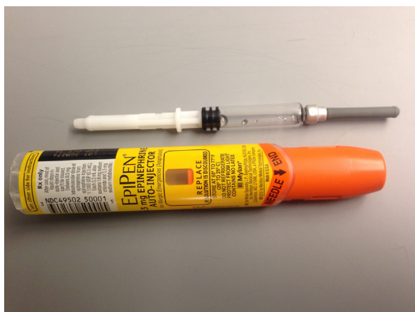
Figure 1. EpiPen autoinjector that has been disassembled to show internal ampule. Solution has been removed.
