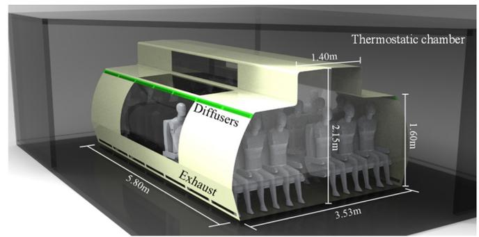
Fig. 1. Schematic of the aircraft cabin mock-up.
