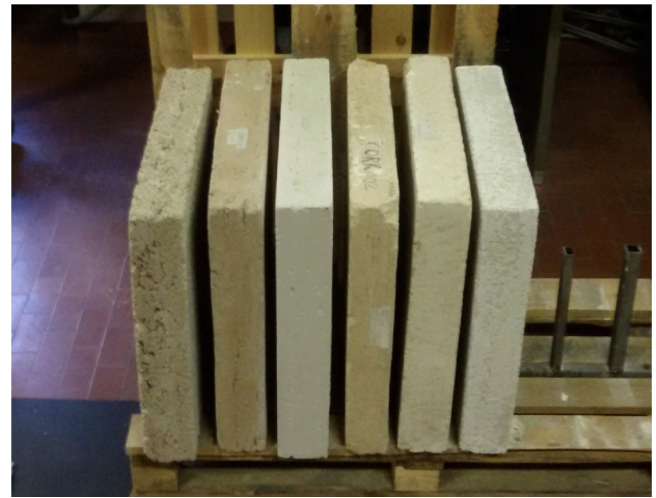
Fig. 1. Plaster samples, from left to right: Bioart cork, VGT.001, Thermocalce, Cork.001, VGT.014, Thermointonaco.
