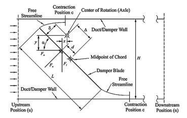
Fig. 1. Schematic presentation of the ATP damper with a single blade [9].
