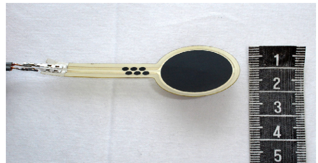
Fig. 1. The force-sensing resistor (FSR) (Interlink electronics, Camarillo, CA, USA) used for the study of pressure (thickness 0.2 \text{ mm} , area 4.15 \text{ cm}^2 ).
