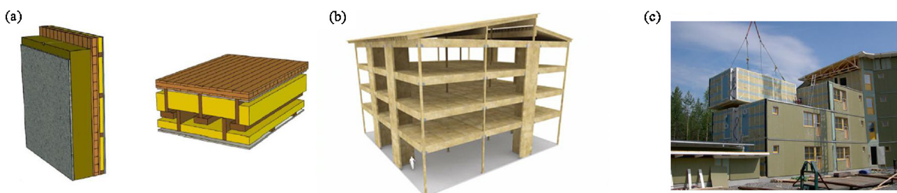
Fig. 2. Photograph and details of some structural elements of the studied building systems including the (a) CLT building system (b) beam -and-column building system and (c) modular volume element building system.
