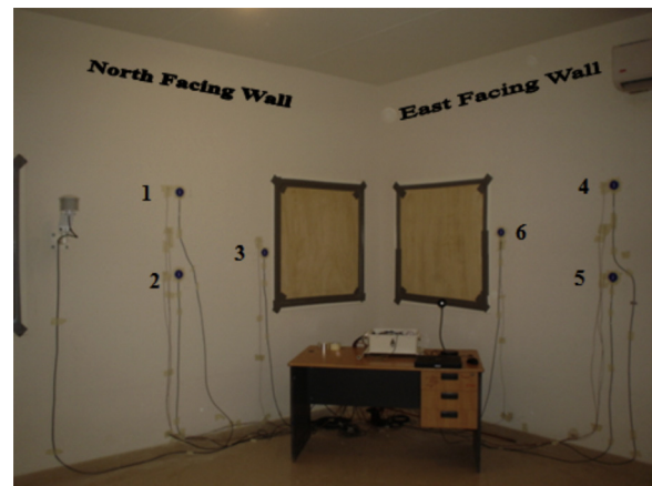
Fig. 2. Inside view of the instrumented walls of the test room.
