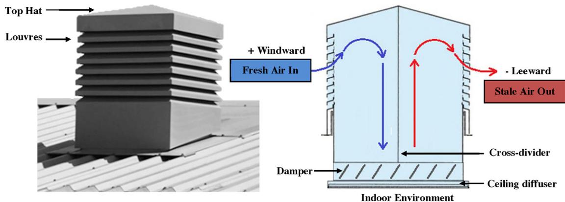
Fig. 1. Schematic of a commercial multi-directional wind tower system.
