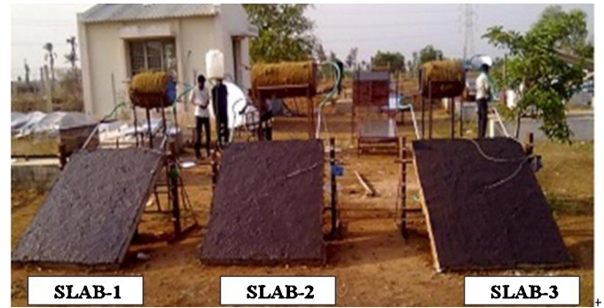
Fig. 2. Concrete slab solar water heating system slab-1 is made up of thermal conductivity materials and aluminium flow pipes. Slab-2 is made up of thermal conductivity materials and PVC flow pipes. Slab-3 is made up of without thermal conductivity materials and PVC flow pipes.
