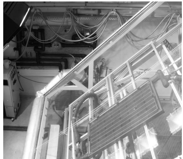
Fig. 3. Picture of the developed prototype during the measurement in the indoor solar simulator.
