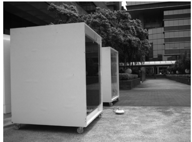
Fig. 1. Outdoor test facility for PV façade (left) and the conventional façade with internal curtain (right).
