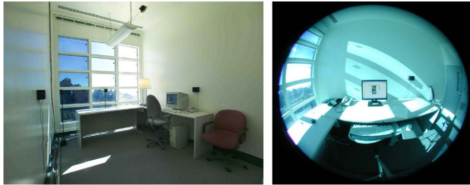
Fig. 1. Perspective (left) and fisheye (right) of test room interior. The left view shows the columns of electrochromic windows at three different levels of transmittance: 5, 30, and 60%. The right view shows the window at 5%. The rooms were not furnished with a task desk lamp (shown in left figure) at the time of the tests.
