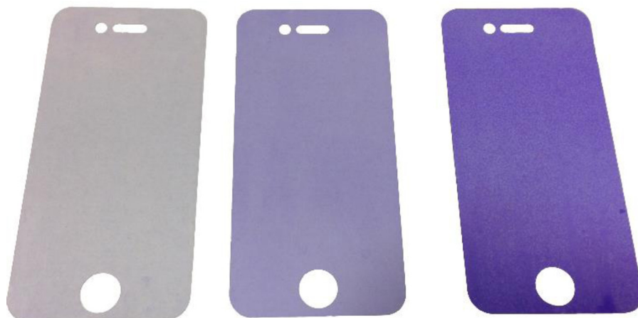
Fig. 2. Dye treated mobile phone screen protector foils, after 5 min, 20 min and 60 min of dye treatment (viewed left to right).
