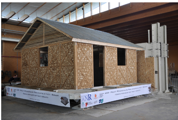
Fig. 2. The house on the shake table.
