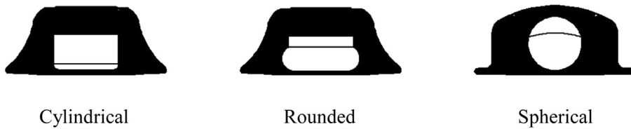
Figure 1. Port chamber shapes. The images are representations only and are not meant to imply exact chamber shapes and/or volumes.
