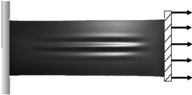
Fig. 1. Stretch-induced wrinkling in sheet – Nayyar et al. [3], permission by Elsevier.
