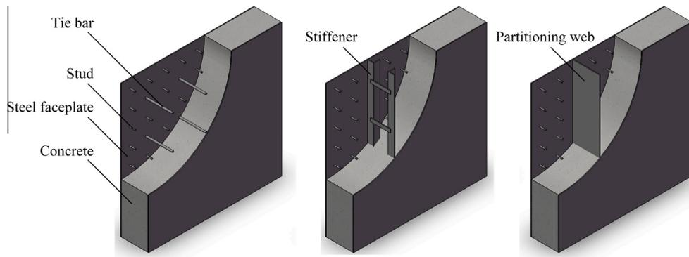
Fig. 1. Typical types of SC walls.
