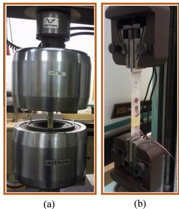
Fig. 1. Tension test setup: (a) GFRP coupons and (b) CS coupons.
