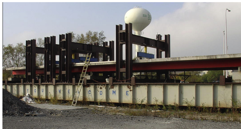
Fig. 1. Overall view of the full-scale two-span, two-lane, continuous prototype bridge.
