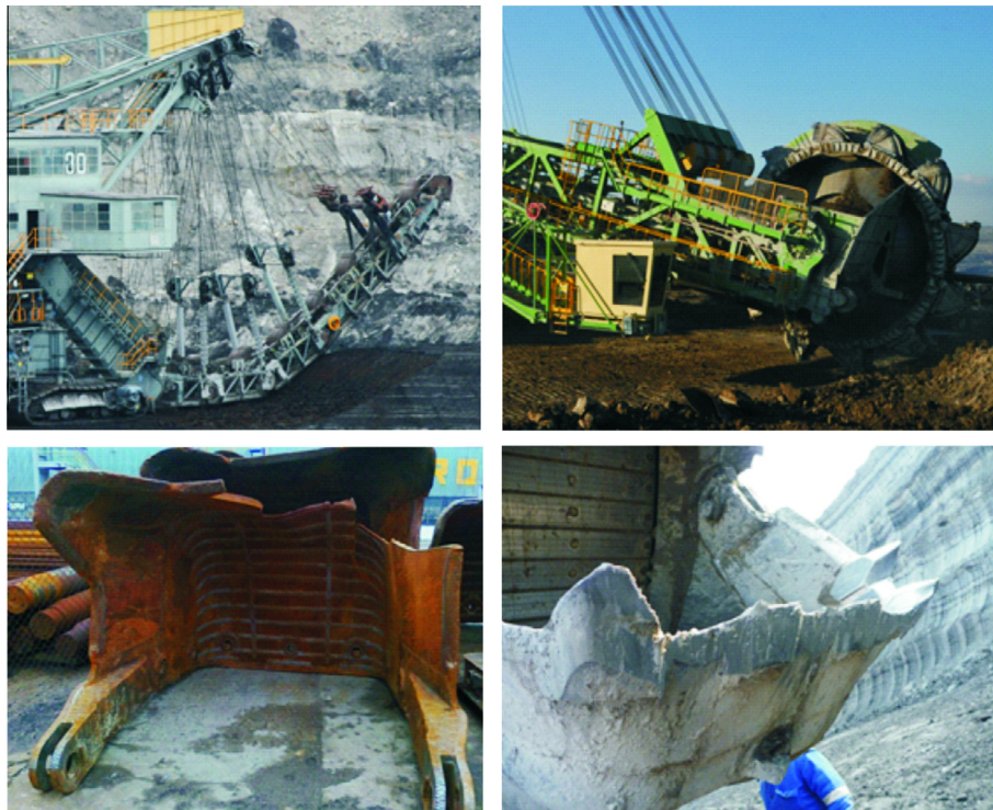
Fig. 1. Excavating units of a bucket chain excavator and a bucket-wheel excavator and examples of wear and damage to buckets.
