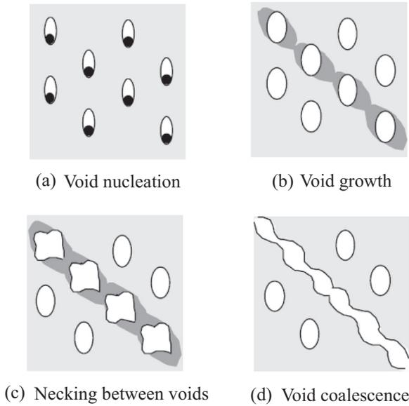
Fig. 1. Mechanisms of void nucleation, growth and coalescence.
