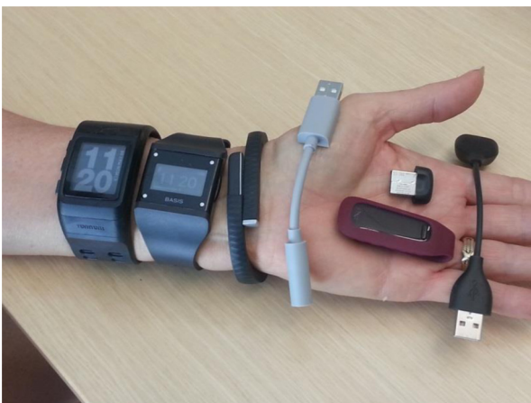
Figure 1. Nike running watch, Basis watch, Jawbone Up with peripheral, and Fitbit One with peripherals.
