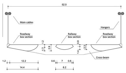
Fig. 2. Geometrical dimensions of the bridge-deck section (m).
