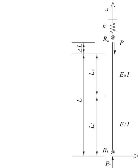
Fig. 2. Column with thermal restraints subjected to non-uniform elevated temperature distribution.
