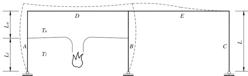
Fig. 1. Steel frame subject to compartment fire.
