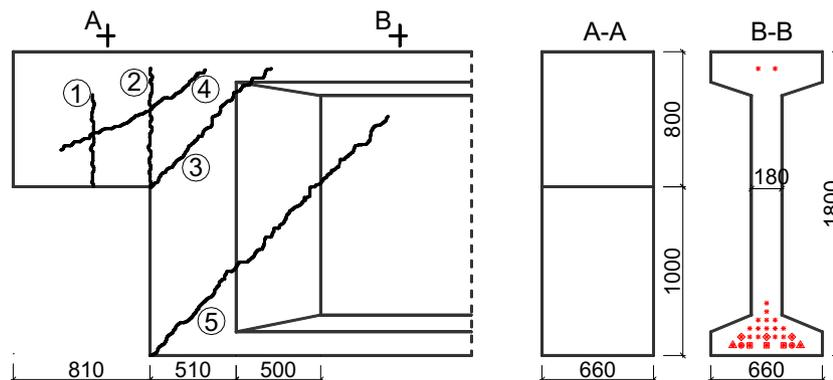
Fig. 1. Potential failure modes in dapped-ends, and cross-sections of the original beams in the real application this study is based upon (dimensions in mm).
