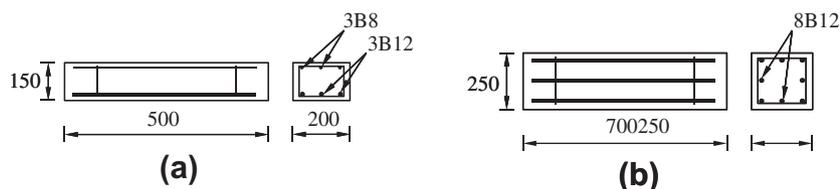
Fig. 1. Corrosion specimens (a) for tension tests (b) for compression tests.
