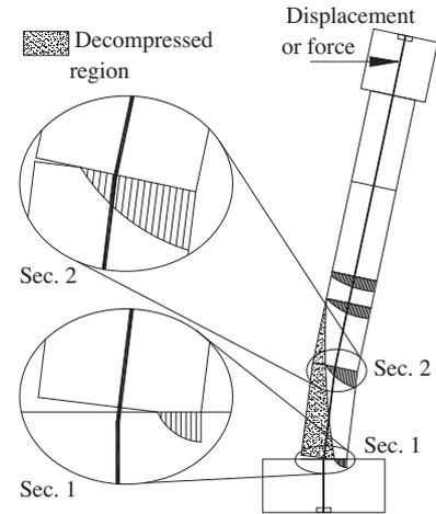
Fig. 1. A schematic drawing of a rocking pier indicating stresses and strains at different heights of the pier.
