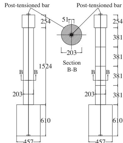
Fig. 2. Schematic drawings of piers FRP1 and FRP4 [mm].
