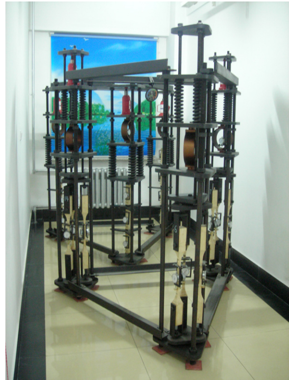
Fig. 1. Test set-up for creep of LVL.
