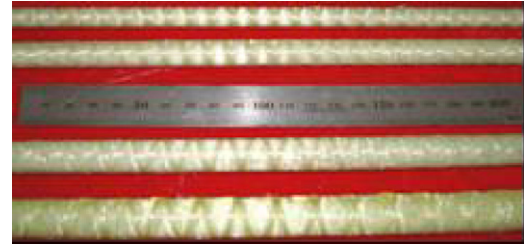
Fig. 2. Surface configuration of GFRP/steel wire composite rebars.
