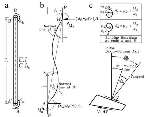
Fig. 1. Beam–column under end moments with semi-rigid bending connections at ends A and B: (a) Structural model; (b) Degrees of freedom, forces and moments in the plane of bending; (c) Rotations at a cross section and at ends A and B.
