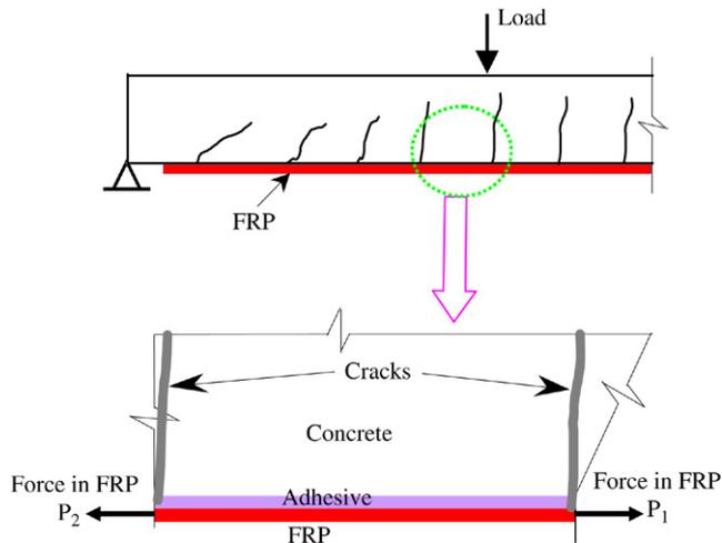
Fig. 1. Intermediate crack-induced debonding in FRP-plated RC beams.
