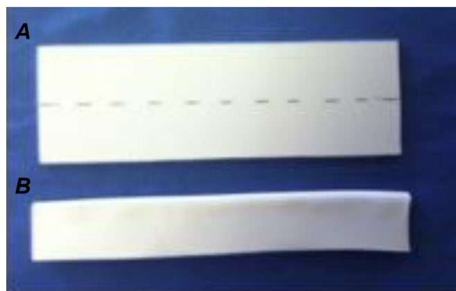
Fig. 1. A. Dotted line across 2" × 6" thermoplast. B. 2" × 6" thermoplast folded into 1" × 6" across the dotted line.
