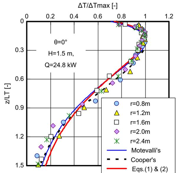
Fig. 1. Typical temperature distribution of ceiling jet at  $\theta=0^\circ$  obtained in small-scale tests.
