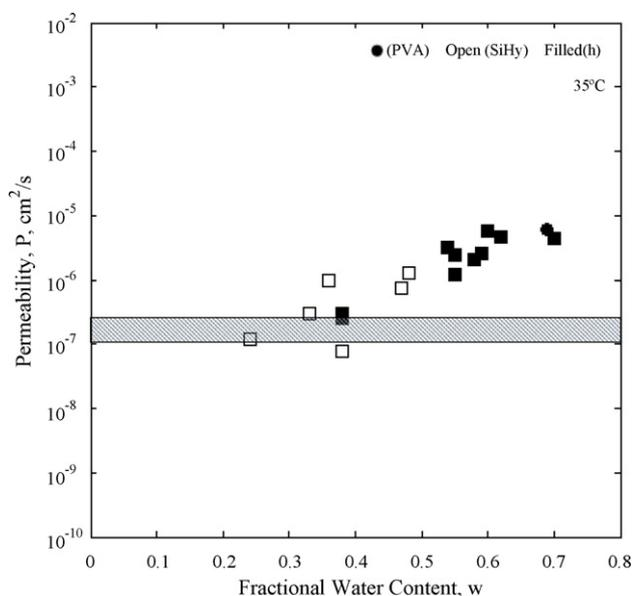
**Fig. 1.** Permeability,  $P$ , of aqueous NaCl in commercial SCLs as a function of equilibrium water content at 35 °C. The filled circle ( $\approx$ ) corresponds to a PVA-based lens (PVA). Remaining filled symbols correspond to HEMA-based materials (H) while open symbols correspond to silicone-based materials (SiHy). The cross-hatched region demarks the threshold permeability for lens movement.
