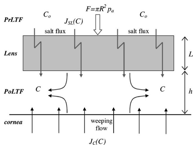
**Fig. 2.** Schematic of the osmotic-withdrawal mechanism for maintaining the PoLTF thickness. Salt diffuses through the SCL with flux  $J_{SL}$ , increasing the PoLTF concentration,  $C$ . Water is drawn through the cornea into the PoLTF by osmotic forces at a volumetric flux  $J_C$ . Drawing is not to scale.
