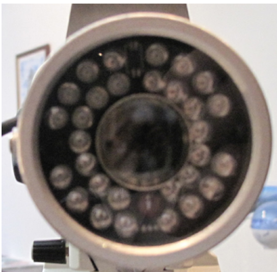
Fig. 3. The portable non-contact IR meibograph (PNCM).
