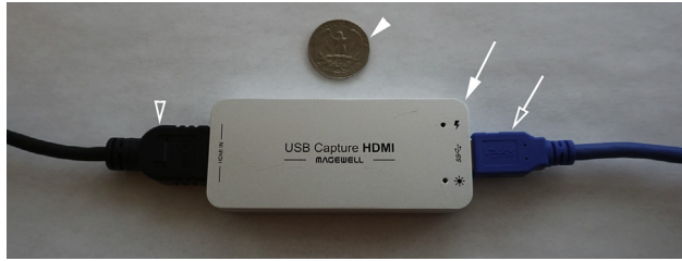
Figure 1. White arrow, universal serial bus (USB) video capture device (Magewell). Void arrow, USB connection to computer. Void arrowhead, high-definition multimedia interface (HDMI) connection to ultrasound machine. White arrowhead, quarter for size reference.
