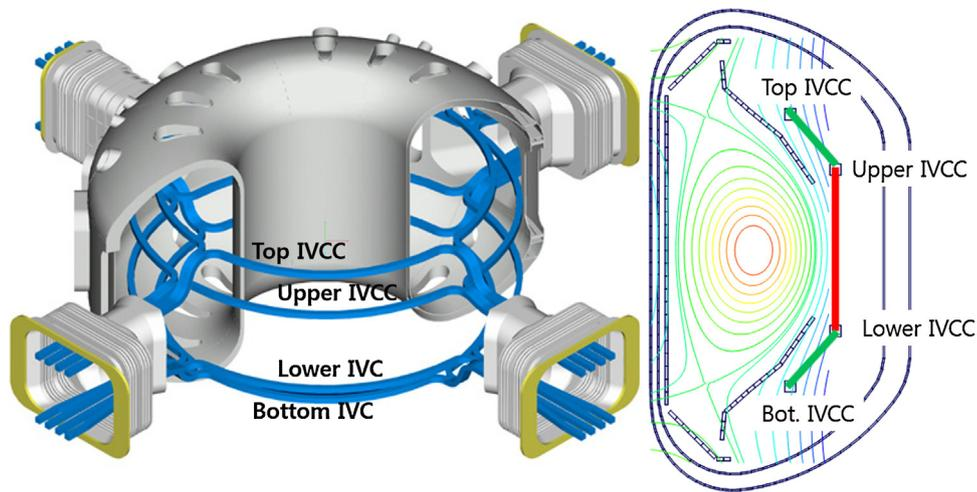
Fig. 1. 3D(left) and cross-sectional (right) views of in-vessel control coils (IVCCs) in the KSTAR tokamak.
