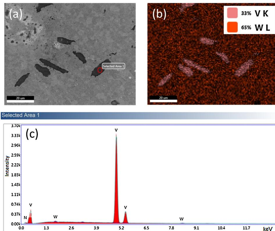
Fig. 1. Phase analysis of the unexposed WVm sample (a) SEM image, (b) elemental map distribution of the same area and (c) EDS of V enriched phase respectively.
