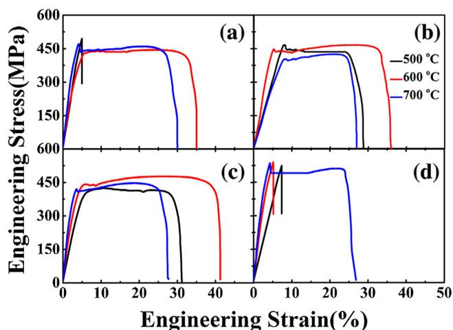
Fig. 2. Stress-strain curves of un-annealed and annealed samples tested at 500, 600 and 700 °C. (a) un-annealed, (b) 1700 °C annealed, (c) 1800 °C annealed and (d) 1900 °C annealed samples.
