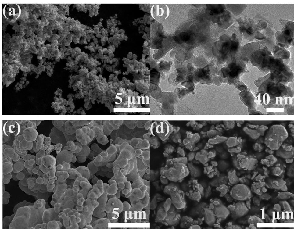
Fig. 1. SEM and TEM images of (a) as-received tungsten powders, (b) raw zirconium carbide powders, (c) raw rhenium powders, and (d) ball-milled powders.
