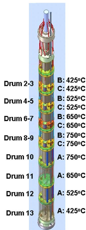
**Fig. 2-1.** Temperatures zones in HIDOBE-01 experiment.
