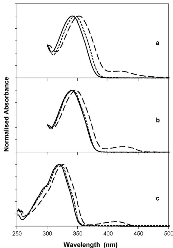
**Fig. 3.** Absorption spectra of (a) esculetin, (b) scopoletin and (c) umbelliferone. For comparison, spectra are normalised at the wavelength of maximum absorbance. Spectra were measured in three anhydrous solvents; acetonitrile (solid line), THF (dotted line) and DMSO (dashed line).
