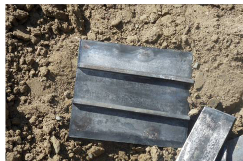
Fig. 3. Welded ribbed single slab after explosive welding in the first stage.
