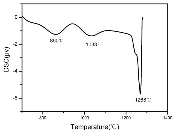
Fig. 2. DSC curve of  $\text{Li}_4\text{SiO}_4$ -Pb pebbles.
