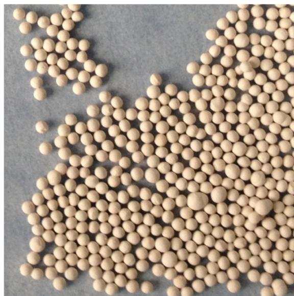
Fig. 1. Macroscopic photos of  $\text{Li}_4\text{SiO}_4$ -Pb pebbles.
