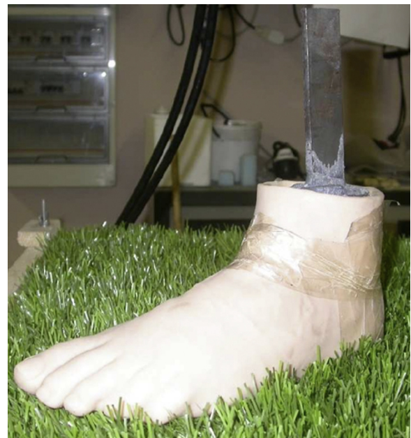
Fig. 2. Artificial foot used in rotational tests.
