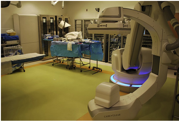
Fig. 1. Hybrid operating room containing Artis Zeego (Siemens Healthcare) robotic C-arm with 3-dimensional imaging capability.
