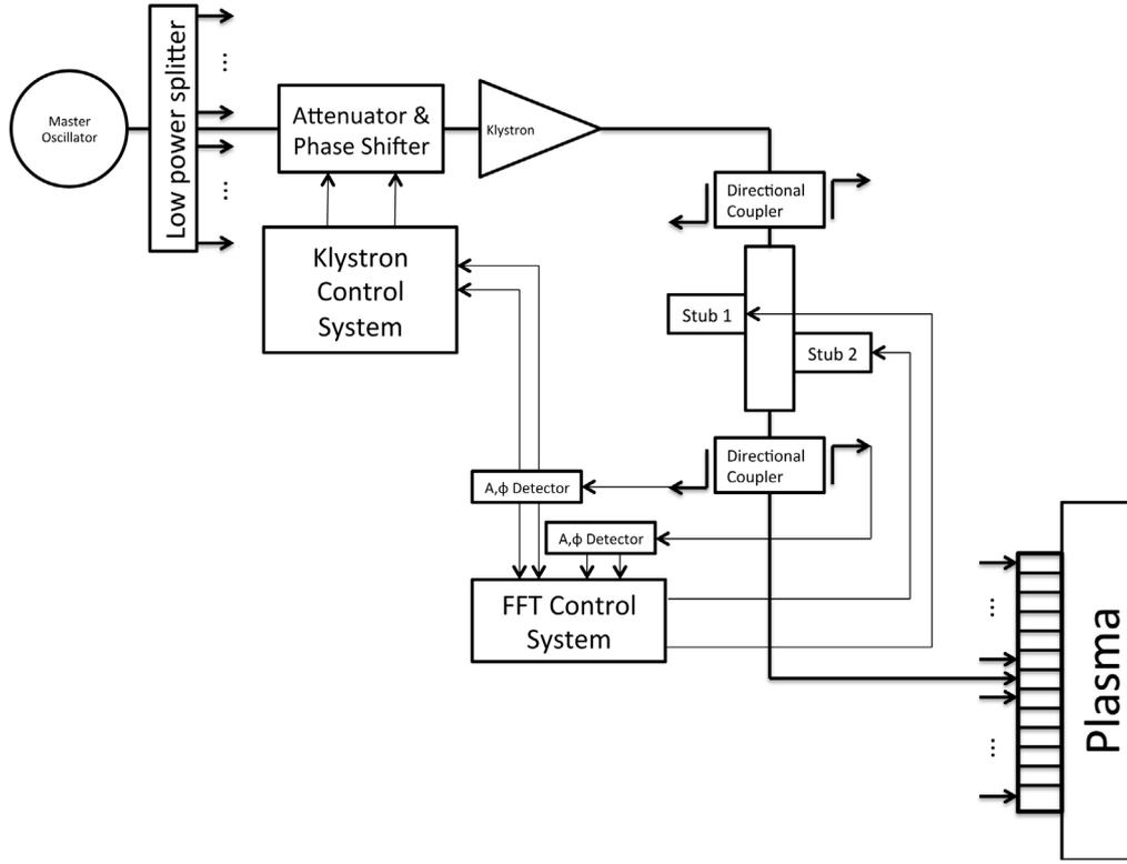
**Fig. 1.** LH FFT system-level block diagram for a single klystron channel, or column. Each column is equipped with an identical system. Two tuning stubs are located between each klystron and the antenna.
